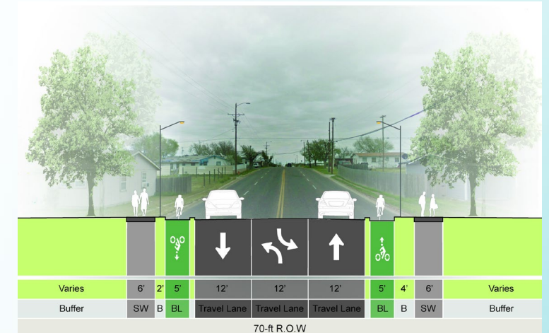
Cross Section with Sidewalk and On-Street Bike Lane
